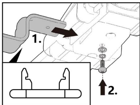
Also the bike carrier must be prepared once for the use of the 3rd bike adapter. Attach the two clamps (3 – 4) to the upper sliding frame of the bike carrier.
