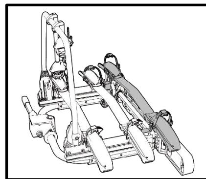
Then slide the 3rd bike adapter in the holders (1) from behind and check if the knobs are secured (2).
